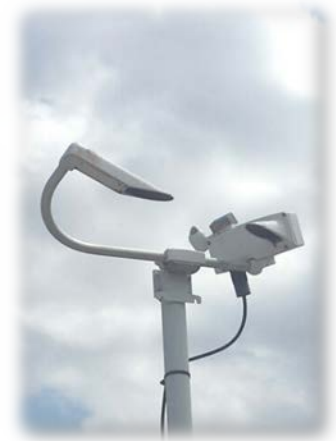
Transmissometer. The instrument on the left fires an infra-red beam to the receiver on the right.
